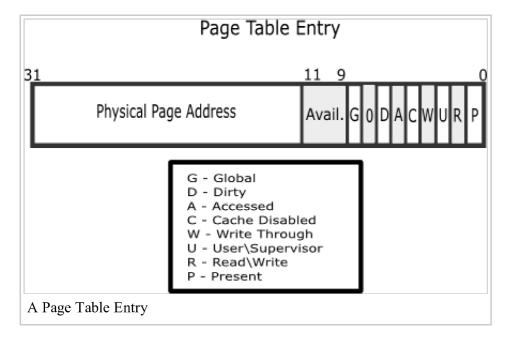
the page global enable bit in CR4 must be set to enable this feature.
